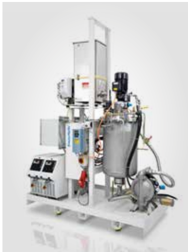
Premixing station for expandable graphite as filler for flame retardant and soundproofing
