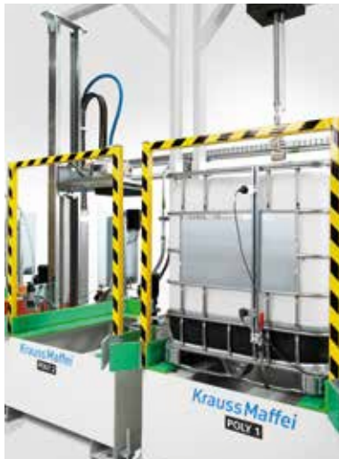
Container station for preconditioning of the PUR components
