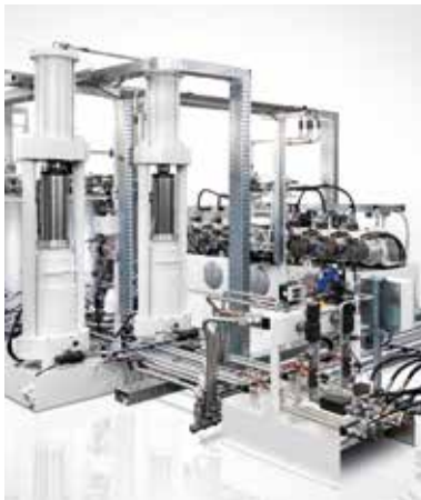
Comet metering machine with hydraulically driven pistons
