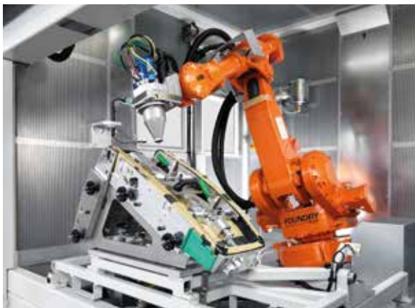
Robotic milling machine for helicopter seats
